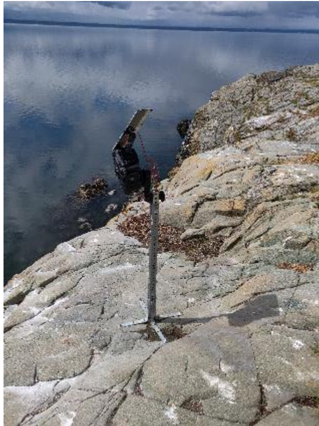
Figure 2-7: The Mitlenatch Island GoPro camera setup (Wilkin, 2021).
